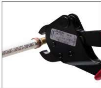
4. Position ring over sealing barbs of the fitting. The ring should be positioned approximately 1/8" to 1/4" from the end of the tube.
