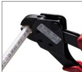
5. Compress tool perpendicular to tubing run. Compress only once. Remove defective connections. Use a gauge to assure a proper joint. Test completed joint.
