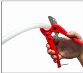
1. Cut tube at 90-degrees. Do not crush OD of tubing with cutters. Hint: Slightly rotate cutter during blade engagement.
